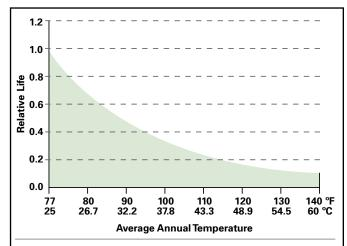
Optimum operating temperature for a VRLA battery is 25°C (77°F). High ambient temperature allows unnecessary large quantities of charge current to flow which results in a shorter service life.
