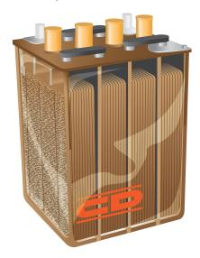
Wet-cell batteries require more advanced maintenance but have a longer battery service life. Like all batteries, UPS batteries are electrochemical devices. A UPS uses a lead-acid storage battery in which the electrodes are grids of lead containing lead oxides that change in composition during charging and discharging, and the electrolyte is dilute sulfuric acid. In other words, they contain components that react with each other to create DC electrical current. These components are:
