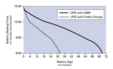
Although batteries are sold with a variety of published life spans, the fact is, some demonstrate a useful life of as little as three to five years. Eaton's exclusive ABM technology significantly increases the life of UPS batteries.
