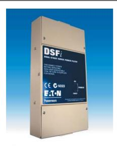
The DSFi is designed to provide secondary protection against power surges caused by external sources such as lightning strikes and substation switching as well as providing a measure of protection from surge events generated on the secondary side of the filter. An ideal device for Category B locations.
